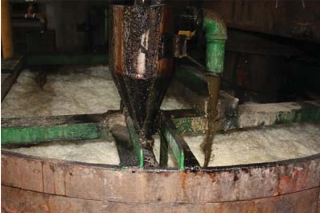
From the clarifying tanks, it flows through evaporating tanks, removing even more liquid.
