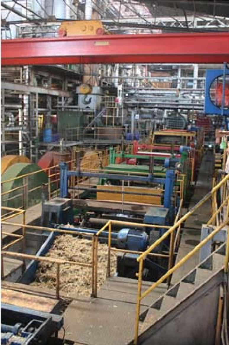
As the cane moves progressively from mill to mill, the pulp becomes finer and drier, until it emerges as a very fine waste product which is recycled in two ways. Part of the pulp is used to make compost which is stacked in a field across the road from the factory, and sold back to the farmers to enrich their fields. Another part is dried and burned to provide energy to help run the mill.
