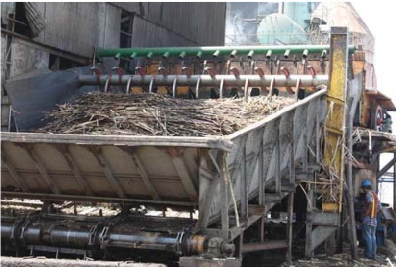
The cane moves up to the top of the feeder where it begins its first process of chopping for the milling process.
