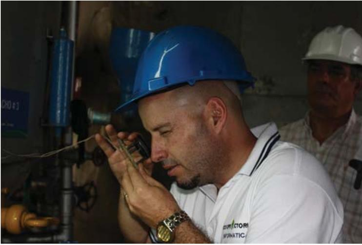
The texture and thickness of the honey is periodically tested by removing a small sample, dripping it onto a piece of glass and checking it with a magnifying glass. The evaporating tanks are very carefully controlled for temperature and timing by computers.
