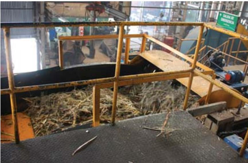
From the feeder on the outside of the building the cane enters the first of five mills where it is chopped finer and finer, each mill pressing the cane with heavy steel and iron drums to extract the juice from the cane.
