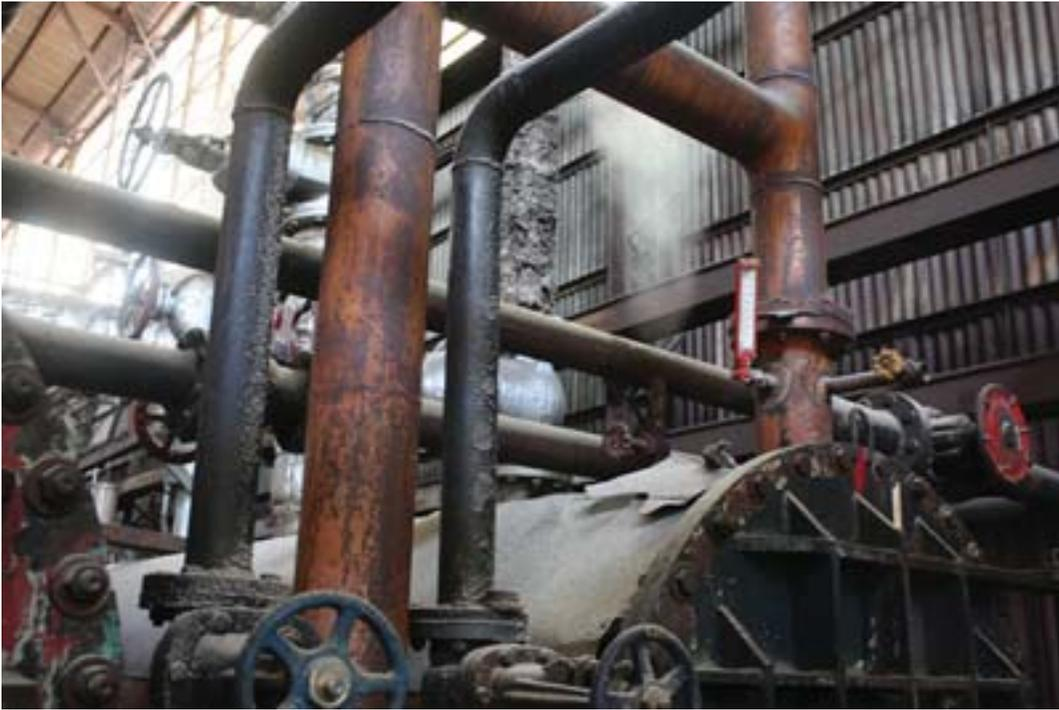
The juice extracted from the cane now begins a series of processes to remove the liquid, remove impurities and reduce the product to the final dry sugar crystals that are packaged and sent to market. First the juice is put into long horizontal tanks where it is heated to extremely high temperatures,
